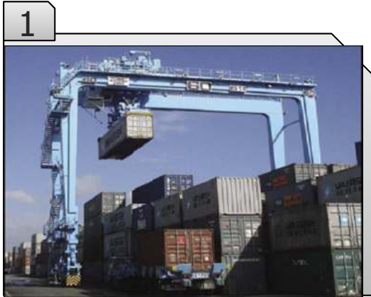
RTGC (Rubber Tired Gantry Crane)
